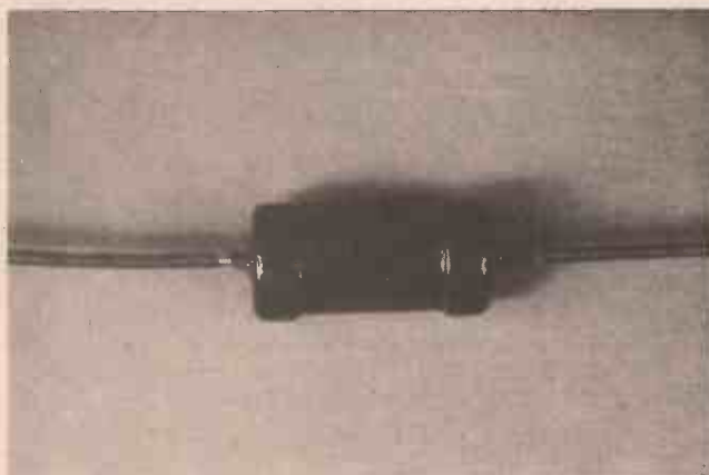
A low resistance wirewound resistor, this type will often find application in power supplies and amplifier output stages.
