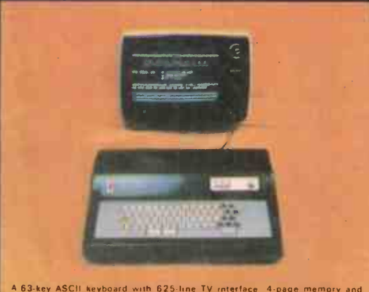
A 63-key ASCII keyboard with 625-line TV interface. 4-page memory and microprocessor interface. Details in our catalogue
