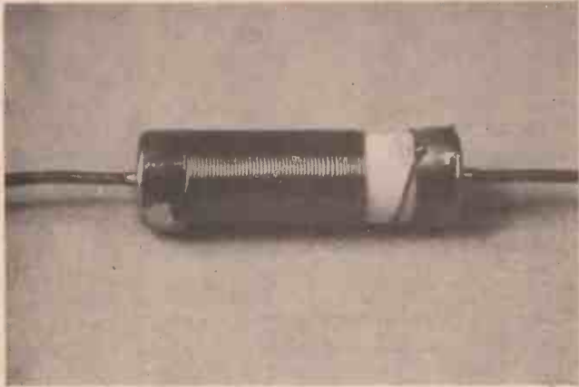
Underneath the skin of a wirewound resistor, a ceramic former is used to aid heat dissipation and electrical insulation.
