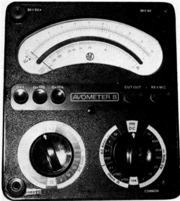
◀ The Avometer is the Rolls-Royce of electronic multimeters. The model 8, pictured left, carries a price tag of over £100.
