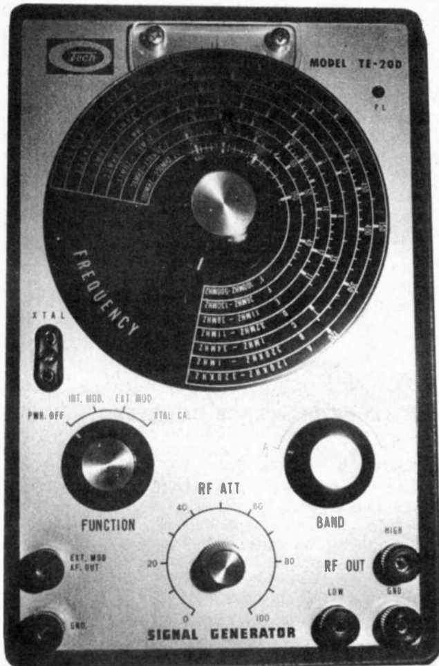
This signal generator will produce frequencies in the range 120kHz to 500 MHz for a price of around £60.
