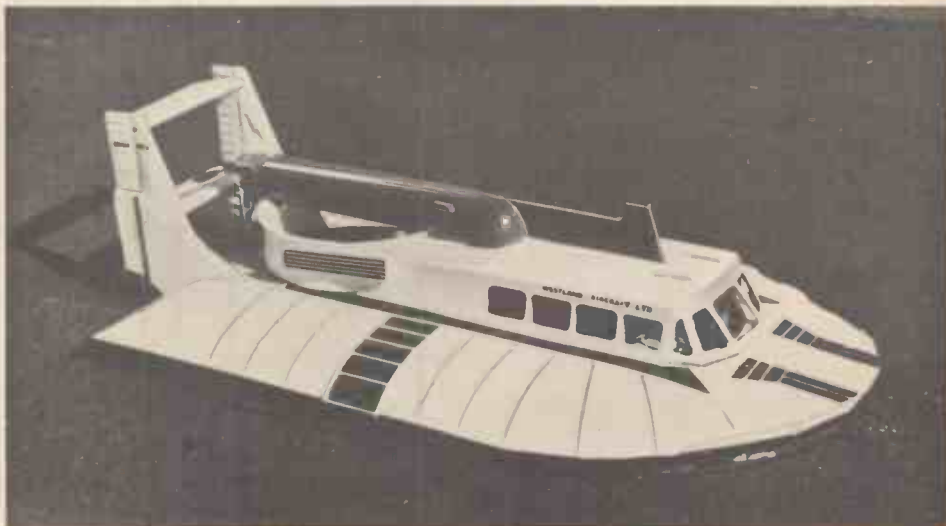
The uses of model internal combustion engines are not confined to aircraft and boats. This scale model Westland SRN-S Hovercraft has two O.S. glowplug engines.
