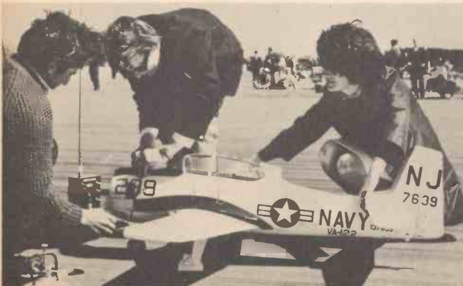
Preparing a radio controlled scale model for flight. This model which has all controls worked by radio including retractable undercarriage, is powered by a 10 c.c. McCoy glowplug engine developing over 1 horsepower.
