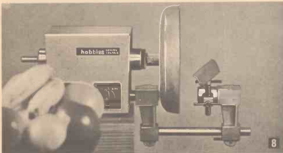
7 WOOD TURNING LATHE KIT DBL. (If parts 129, 131 and 1311 of kit CEW. 4 already exist). For work up to 5½ in. approx. (140 mm.) diameter, 16 in. to 36 in. approx. (400 to 900 mm.) in length. Universally adjustable chisel support, centre running on ball bearing, three prong chuck. Complete with turning chisel. (Consists of parts 133, 134 and 135).
