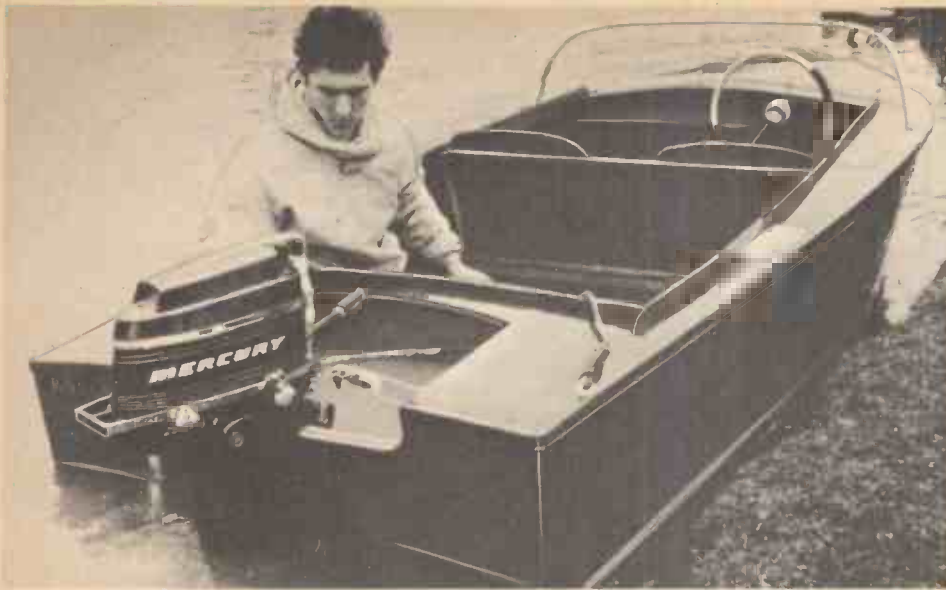
The complete boat afloat. There is remote steering, windscreens, mooring cleats and steps on the side decks.
