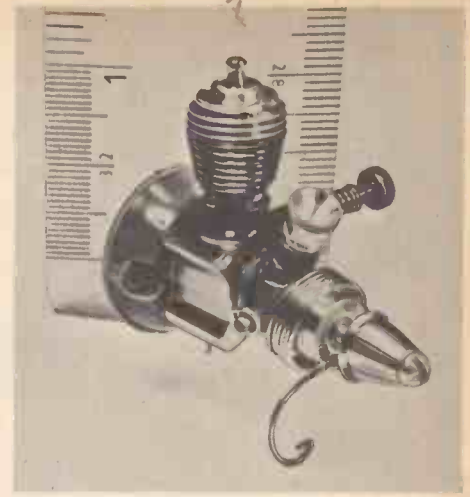
The World's smallest model internal combustion engine. The remarkable little Cox 'Tee-Dee 010' motor has a piston diameter of less than \frac{1}{16} in., and weighs \frac{1}{2} oz.
