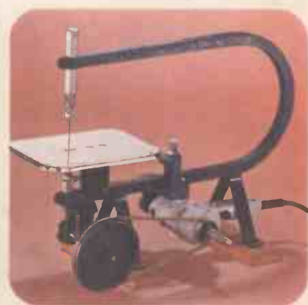
The Hobbies 'Marvel' fretsaw machine with electric motor. See page 90.
