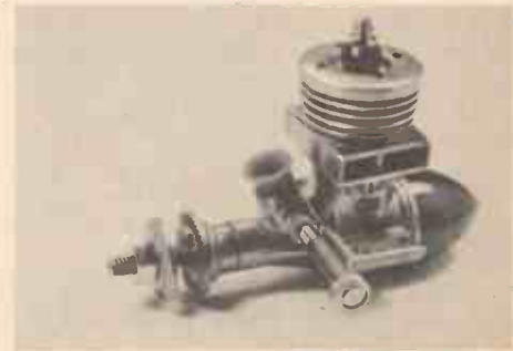
Another low-priced engine suitable for the beginner, the 'Fuji 099' glowplug motor of 1.6 c.c. capacity.
