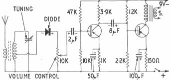
Fig. 41-Transistor receiver circuit
