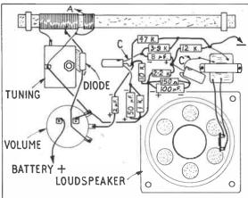
Fig. 42—Wiring plan of the receiver
