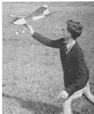
Launch the model smoothly with nose pointing downwards.
