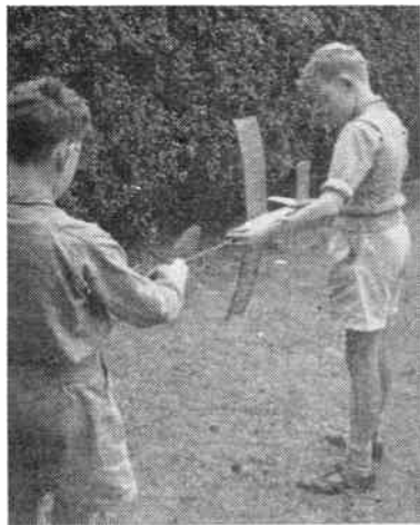
Method of winding the motor, showing how the rubber is 'stretched' from the fuselage during winding.
