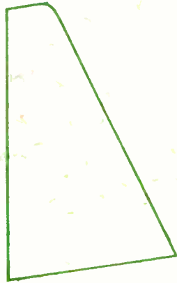
STRUT. CUT ONE 1/4in. (ONE FOR EACH CALENDAR).
