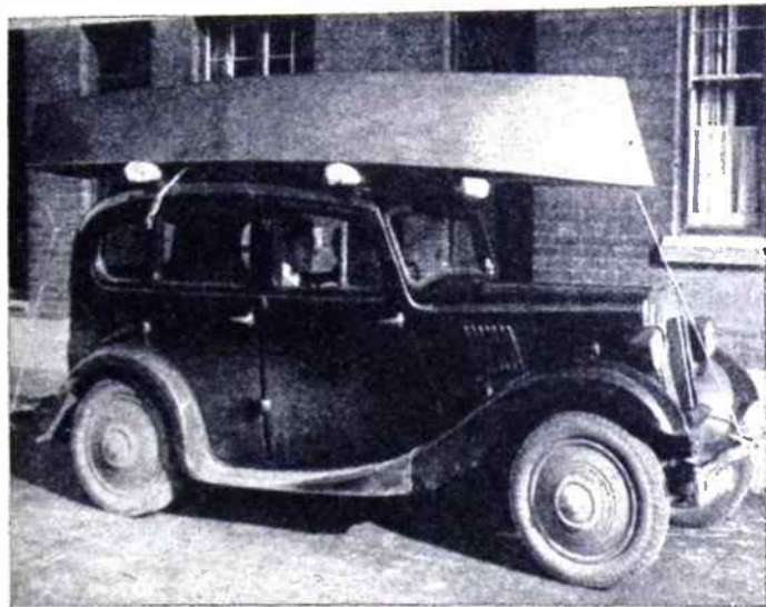
This 11 ft. fishing dinghy can easily be carried on the roof of a small car. Note the simple 'slabsided' construction. Such a craft would be rather too sluggish to sail
