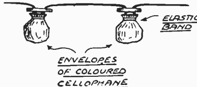
Quick way of colouring small battery-run bulbs
