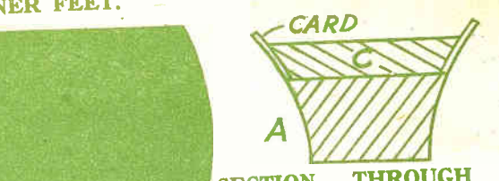
SECTION THROUGH KEEL ON LINE A.A. SHOWING HOW THE UPPER SIDE, MADE OF CARD, IS GLUED TO PIECE C, TO COME FLUSH WITH KEEL. PIECE A.
