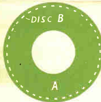
DISC AT END OF RECEIVER. CUT ONE 3 16in.
