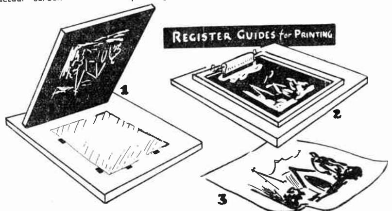
(1) Screen raised, with stencil mounted, and job in register on baseboard. (2) Screen lowered and squeegee ready to draw across the screen to force colour through mesh. (3) The finished print in one colour
