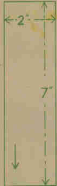
FLOOR. CUT ONE 3 1/4 in. TO SIZE SHOWN
