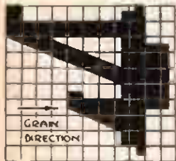
Wooden bracket shapes, plotted in \frac{1}{4} in. squares
