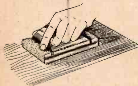
Fig 1—Use glasspaper flat on a block
