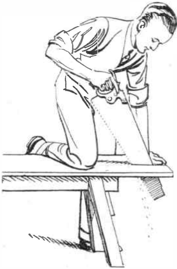
The position for ripping down a board
