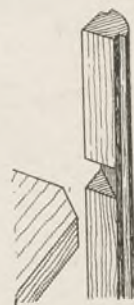
Fig. 4—Fitting the bottom in the leg
