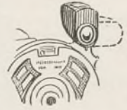
The Folding Camera view-finder with changeable position
