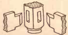
Fig. 2.—The ends of the tenons must be chamfered off so they meet and bed together in the mortise in the leg.
