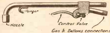
Fig. 1.—The gas blow-pipe.
