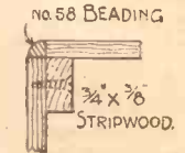
Fig. 3.—Looking down on the corner to show sides, the fillet strip, and the corner decorative beading.
