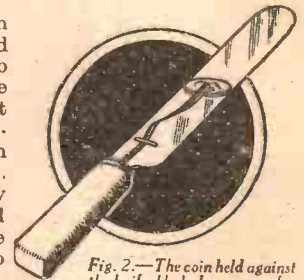
Fig. 2.—The coin held against the knife blade by means of a spring catch.
