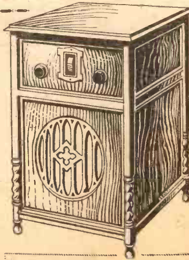
This compact instrument contains the set and speaker, can be made for gramophone amplification, and used as a table. Quite simple and cheap to make in oak.
