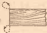
Fig. 4.—Ensure a sharp corner on the pattern by cutting round in the waste wood.
