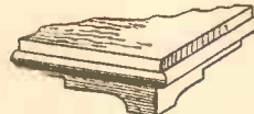
Fig. 4.—Two pieces of fretwood the shape of the one above make an excellent corner foot if fitted as shown in the lower illustration.
