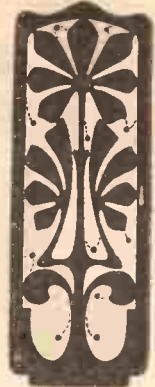
Fig. 9.—A pattern showing the best place for the drill holes. The dotted lines indicate the commencing direction of the saw.
