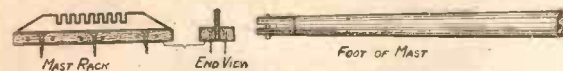
Fig. 5.—The pin shown at the bottom of the mast drops into slots in the mast step-rack.
