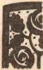
Fig. 8.—Two or three holes can be made in each pattern to be cut; it facilitates the turning of the saw.
