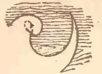
Fig. 6.—Another corner where the saw turns in the waste wood to approach properly.
