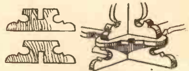
Fig. 5.—An ordinary fretwork foot, made in two pieces and fitted together by the halving joint. This forms a rigid and flat corner for almost any article.
