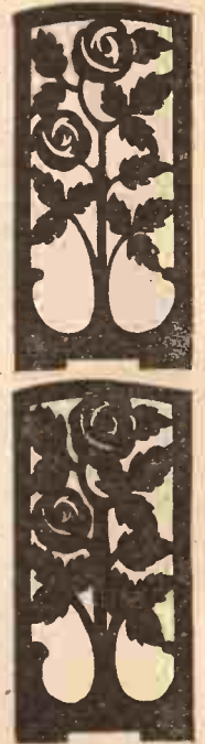
Fig. 2.—The result of cutting with a sloping saw. Above is a correctly cut design; below is the same pattern on the underside.
