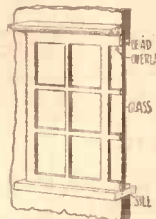
Fig. 2.—The window broken away to show the various parts in it.
