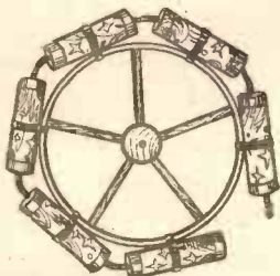
A large wheel. When ignited this spins round emitting a coloured circle of fire. The first firework, when finished, fires the second one and so on round the circle.
