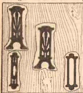
Fig. 6. Above is an example of wasting wood by putting the designs on anyhow.
