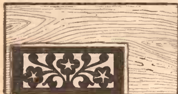
Fig. 5. Paste the straight line of a pattern along the edge of the wood to save having to cut it. A very useful hint.
