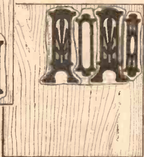
Fig. 6. Below you see the way to paste patterns as closely together as possible to save wood.
