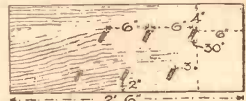
Fig. 3. A plan of the sides giving the position of the racks and the various dimensions to mark off for cutting.
