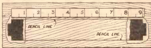
Fig. 8 (Below). The same design as it is pasted to the wood. The two parts are stretched to the dimension printed and joined by pencil lines.
