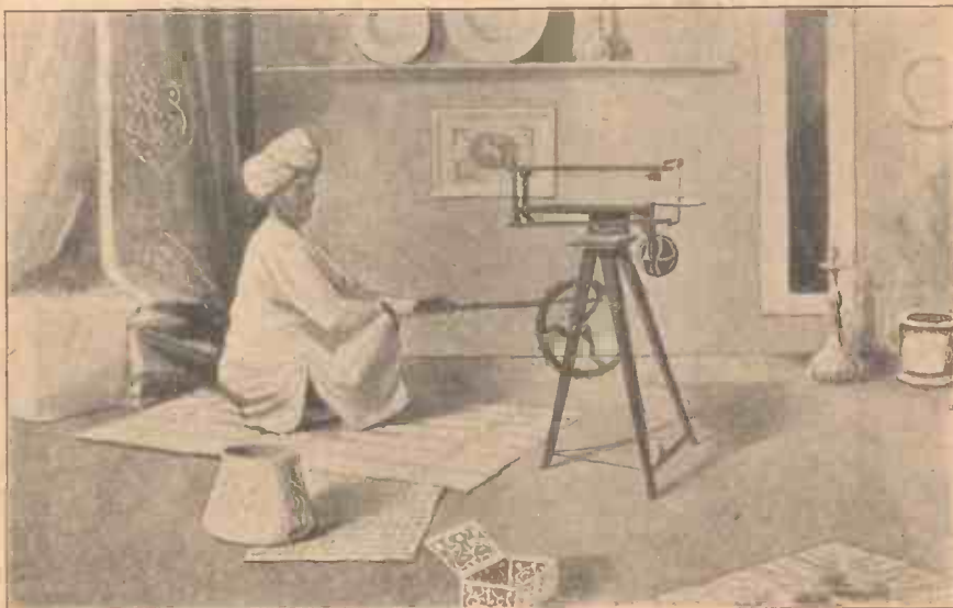
TREADLE FRETSAW "POWER ATTACHMENT" IN INDIA.
