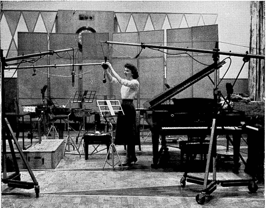
It often pays to set up the microphones in their approximate positions before the musicians assemble (BBC photo)
