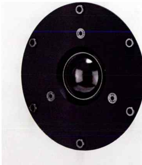
The 770's 28mm microfibre dome tweeter with back damping to suppress resonances in the acoustic chamber. Being large it goes low smoothly.
