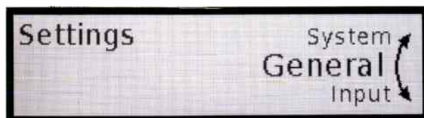
A sensibly-designed user interface, which takes advantage of a readable LCD panel. From here, you can configure inputs, volume levels and standby button/headphone behaviour amongst other things. The display also indicates sampling rate when the Pre-XR is in DAC mode.
