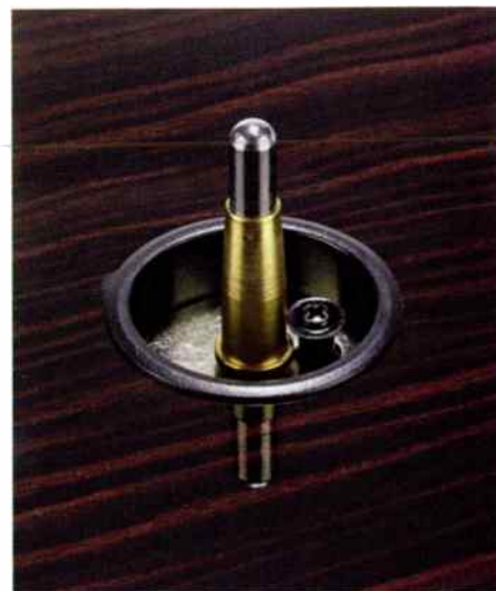
The bearing has a brass taper to grip the alloy platter. The shaft is tightly machined for little play, contributing to speed stability.
