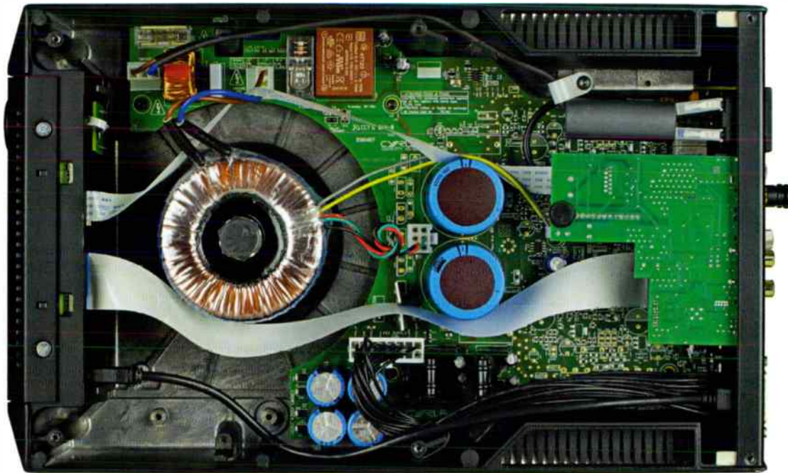
Inside the Pre-XR. The QXR DAC module is clearly visible to the right of the picture. Underneath it, on the motherboard, are the phono stage, volume control and input-switching relays. Cyrus has specified a linear power supply, as evidenced by the toroidal mains transformer.
