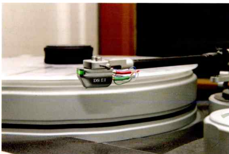
DS Audio DS-E1 optical cartridge that comes with special pre-amplifier with power and equalisation unique to the cartridge.
