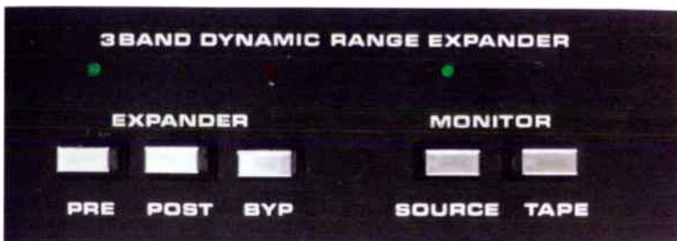
'Pre' and 'post' buttons retrospectively determine whether the deck's input or output is expanded; in the former mode, the corrected signal is recorded. The bypass button allows the replay signal to be expanded.
