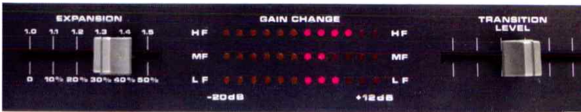
Sliders control the level of expansion - from 1.0:1 (none) from 1.5:1 (50%) - and the 'transition level'. This is the point at which lower signals are made quieter, and higher ones louder.
