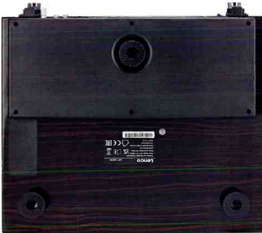
A large plastic cover hides the phono stage, control electronics, USB stage and Bluetooth transmitter. The three feet are not height adjustable so a flat surface is needed.
