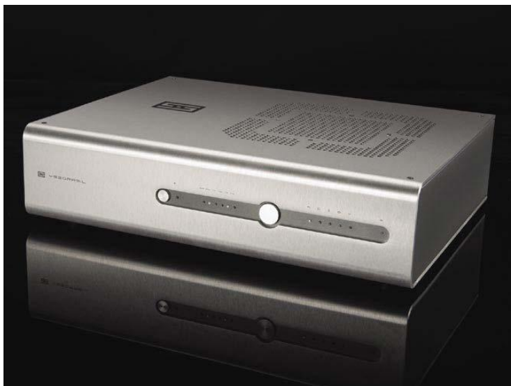
The ShiiT Yggdrasil CD player uses their r2r resistive ladder digital convertor (DAC), making it substantially different.
