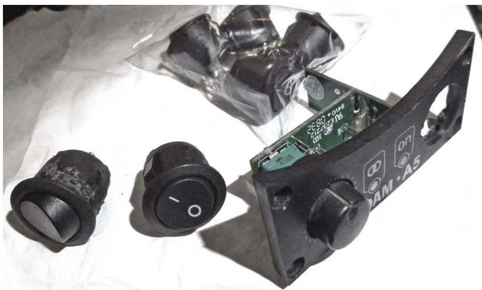
Adam's choice of front-panel mains switch alas tends to fail after several years of use, leading to dead or permanently-on speakers. Fortunately, exact replacements for these single-pole switches are cheap to buy on eBay. Bridging a dead switch's contacts is however a cheaper alternative.
