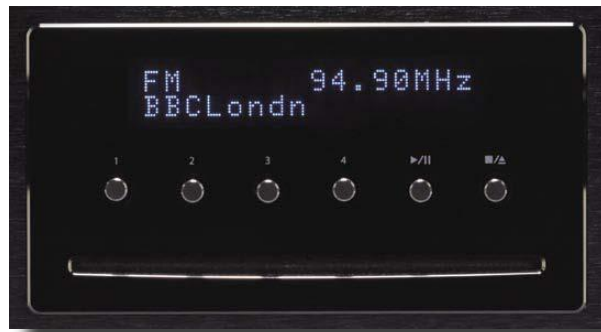
The blue dot-matrix display gives basic information only, but is visible at a distance. Forty presets can store station frequency, for instant selection.
