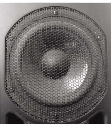
The 5.5 in midbass driver, which crosses over to the tweeter at 2.2kHz, is protected by a metal grille. Its cone is made of an unusual composite material – a sandwich of Rohacell (described as a "lightweight structural foam") and carbon-fibre. Although it doesn't go particularly low, the A5's bass is tight and accurate.
