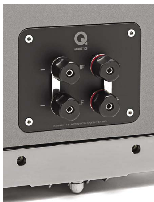
Sturdy bi-wire terminals sited low down at rear, fitted with links for conventional mono-wiring. The links must be removed for bi-wiring, where separate bass and treble cables are used.
