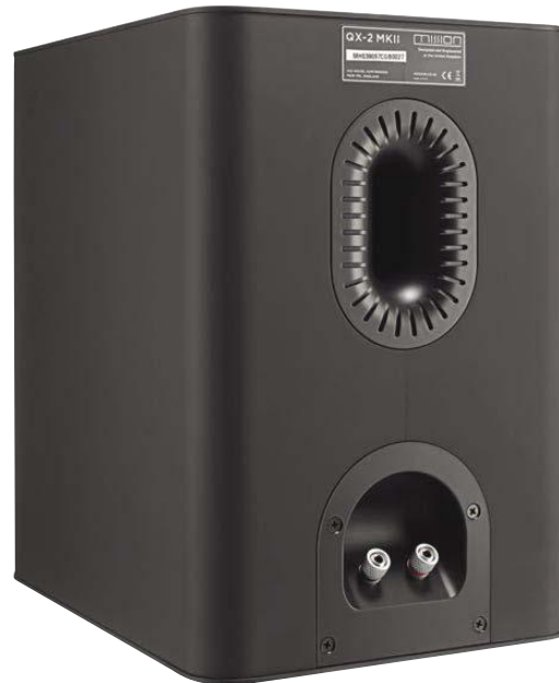
An unusual rear port with serrations to improve air flow, Mission say. Tuned to 40Hz it also helps the small 'speaker go low – right down to 30Hz our measurements show.
