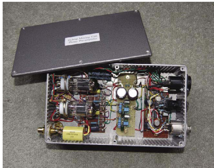
David Lord's hybrid phono preamplifier, using an LM394 front-end and ECC83 double triode output valves. External power supply not shown here.
