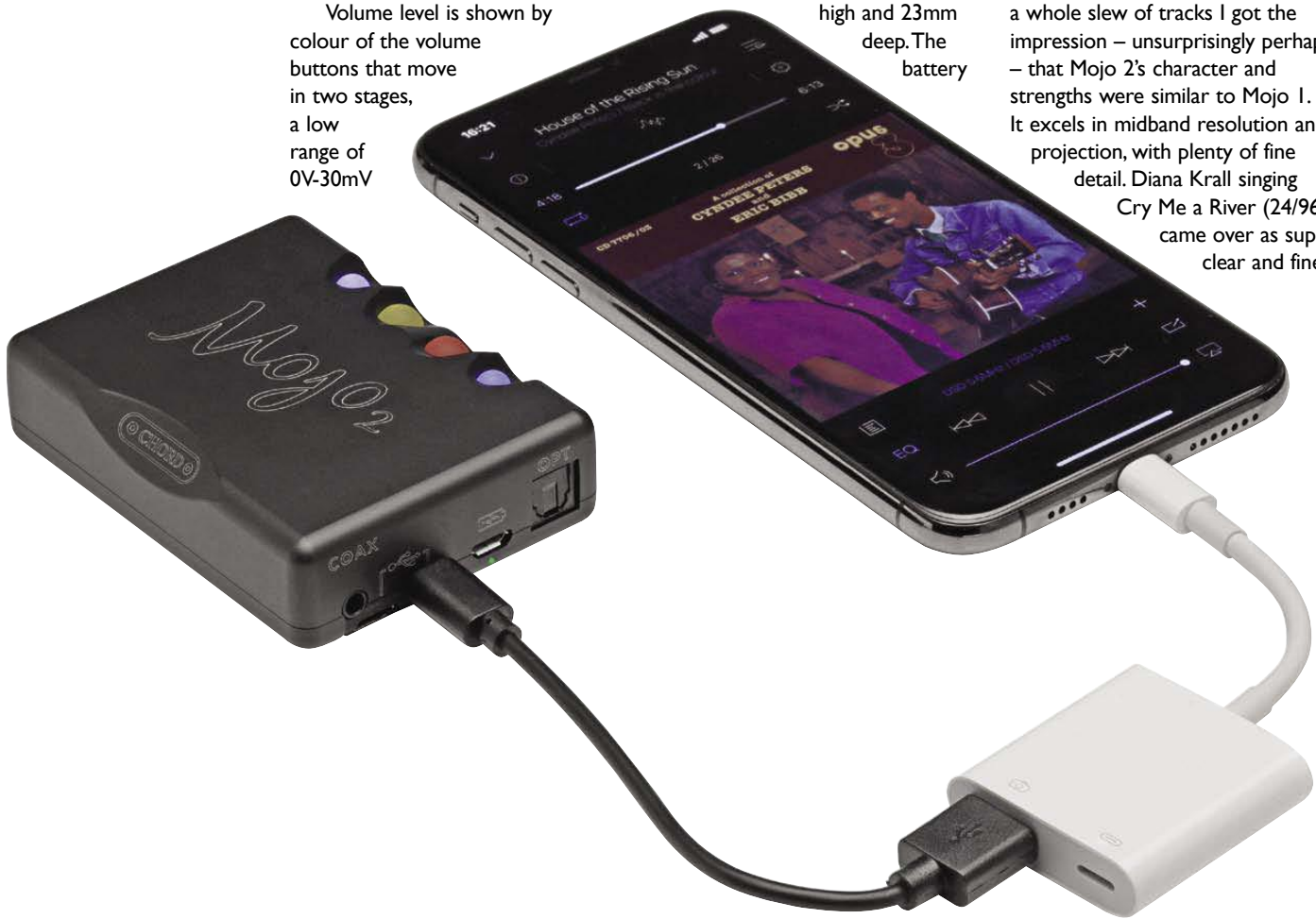
Connection to an iPhone is through an adaptor; a direct Lightning-to-microUSB cable does not work we found. Here an Onkyo HF player app for iPhone sends House of the Rising Sun (DSD) out to Mojo 2 – and not as PCM since Mojo's indicator (the power button) lit up white, as shown here.
