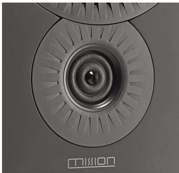
Mission's ring-dome tweeter – an annular diaphragm that forms a ring, driven by a voice coil. At centre lies a static phase plug to break up cancellations across the diaphragm. Ring domes are more complex than traditional domes but give smoother response by avoiding cavitation of dome apex.
