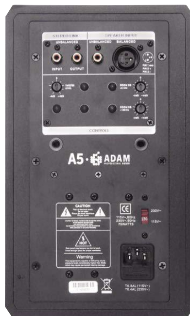
Plenty going on here – these are professional workhorses, not consumer hi-fi equipment. As active speakers, the A5s can be fed at line-level via phono sockets (unbalanced) or XLRs (balanced). Low and high levels can be adjusted to compensate for room acoustics.
