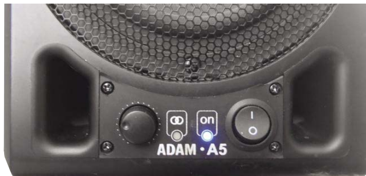
Just beneath the woofer are the volume control and that trouble-prone mains switch. In addition to a power-on LED is one that illuminates when the 'stereo link' mode is active.
