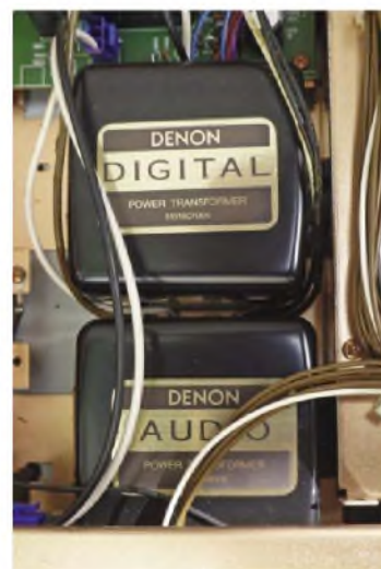
A heavyweight resonance-damping copper chassis, and a linear power supply arrangement based around two transformers, contribute to the DVD-5000's 17kg of high-end DVD goodness.
