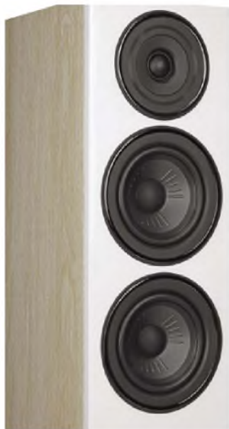
The two bass/midrange drive units have ribs to add stiffness and break up waves. The black cone material is a polypropylene/mica composite.
