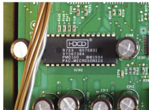
The DVD-5000 can play 'pseudo 20-bit' HDCD titles – remember those? – thanks to a genuine Pacific Microsonics PMD100 decoder chip. Even if its DVD loader no longer works, HDCDs can be spun on a transport feeding one of the DVD-5000's digital inputs.
