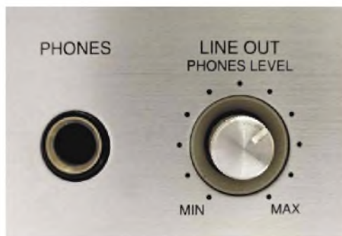
The DVD-5000's headphone amplifier is surprisingly capable, and can drive decent headphones. Its level control also affects the rear-panel 'variable' output.
