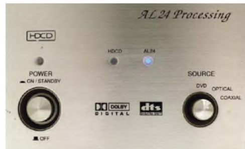
A front-panel knob switches between the internal transport and the two inputs (optical and digital). Also visible are the LEDs that indicate when the DAC is upsampling 16-bit material (AL24) or decoding HDCDs.
