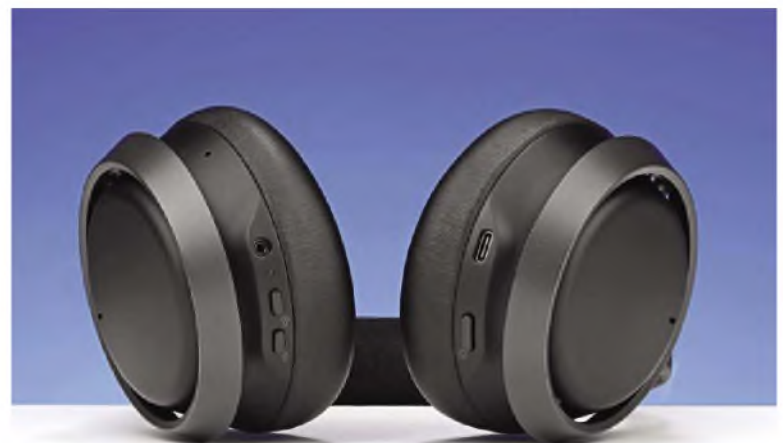
The Right earpiece carries a 2.5mm stereo input jack, ANC and Mic buttons. The Left earpiece carries a USB-C 5V charging socket and on/off button.
