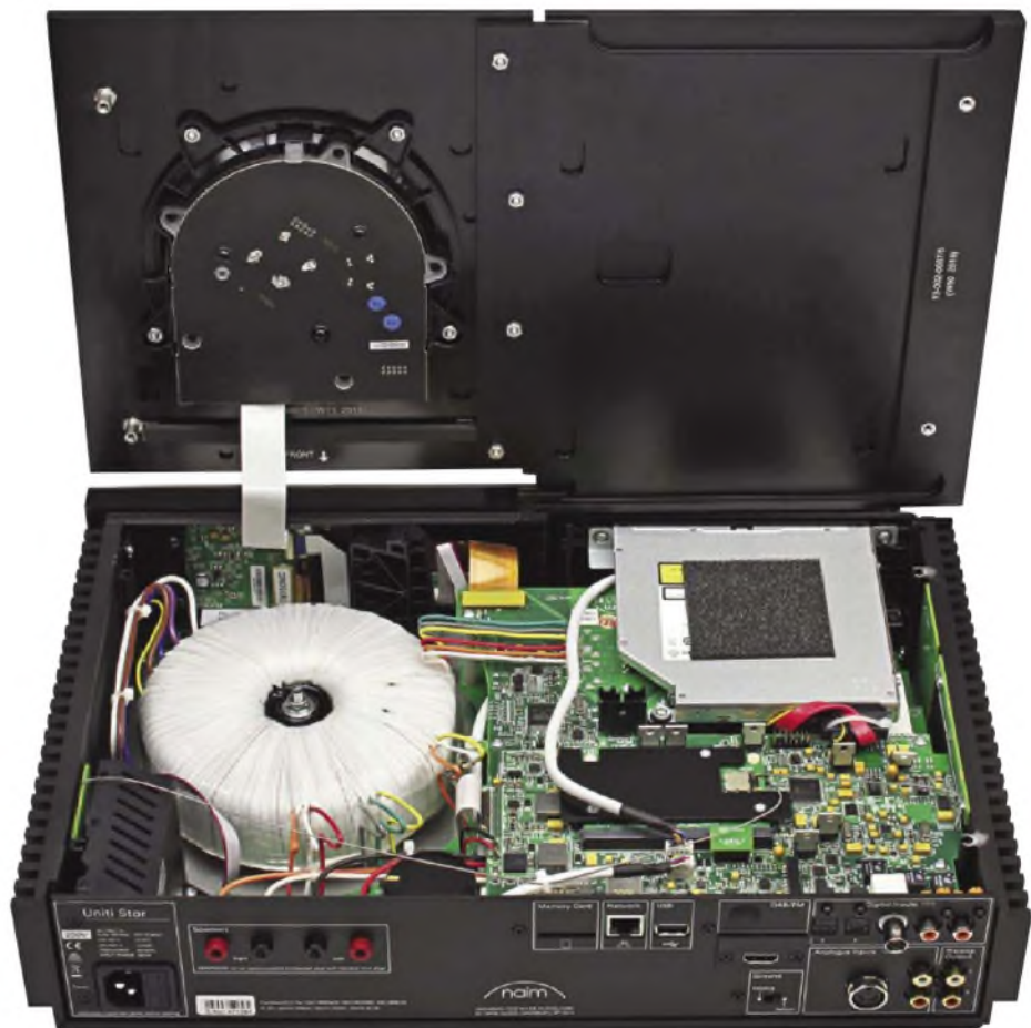
Internally the Uniti Star is dominated by a massive toroidal mains transformer (left). At top right is the CD transport. Around these large components sits a complex array of electronics.
