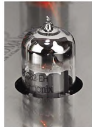
An ECC82 EH double-triode preamplifier tube from Electro-Harmonix.
