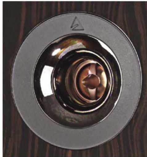
The magnesium dome tweeter comes with a combined phase plate/plug assembly to control output, buried in a short horn to project energy forward.
