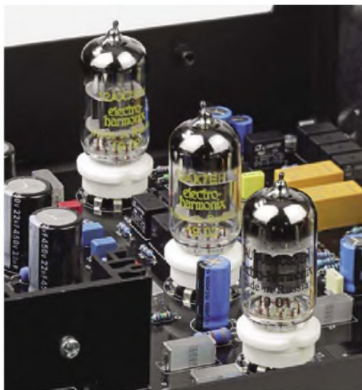
Two Electro Harmonix 12AX7 (ECC83) double-triode preamp tubes and one ECC82 (12AU7) cathode follower output tube provide amplification for MM cartridges. JFET transistors provide further amplification for MC cartridges.
