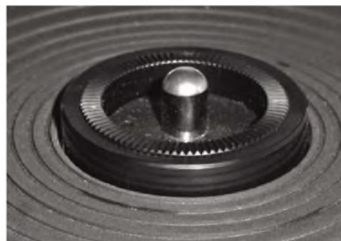
The SL-7 - like the SL-10 - has a 'pop-up' 45rpm adaptor. Note that the platter mat is fixed so cannot be replaced.
