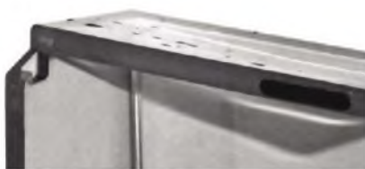
The fragile lid catches can break if not treated with care, then the lid won't close properly. To minimise the risk of reducing the deck to this state, the latching system must be used carefully.
