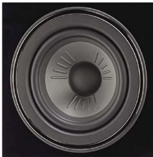
Wharfedale's proprietary Klarity cone material is lightweight yet rigid and further stiffened with raised ribs. The low-damping surround is designed to minimise colouration and improve dynamic expression.
