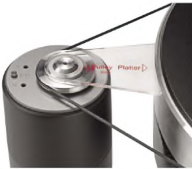
An clear plastic alignment guide locates the free standing motor relative to the platter, imposing a spindle-to-spindle distance of 214mm.
