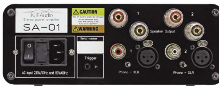
A master power switch at left and solid gold-plated loudspeaker sockets at top. The balanced XLR inputs are standard, the gold plated phono socket inputs an extra, selected by toggle switch.
