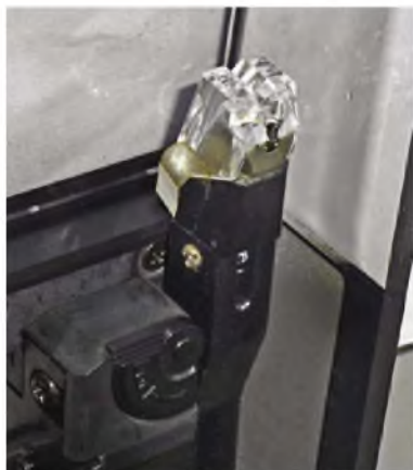
Technics fitted the SL-7 with an EPC-P202 MM P-mount cartridge with a boron cantilever, fitted with an elliptical diamond tip. Technics was one of the first manufacturers to adopt the T4P 'P-mount' pluggable cartridge system, which is still supported today. The arm-lock lever is also visible here.
