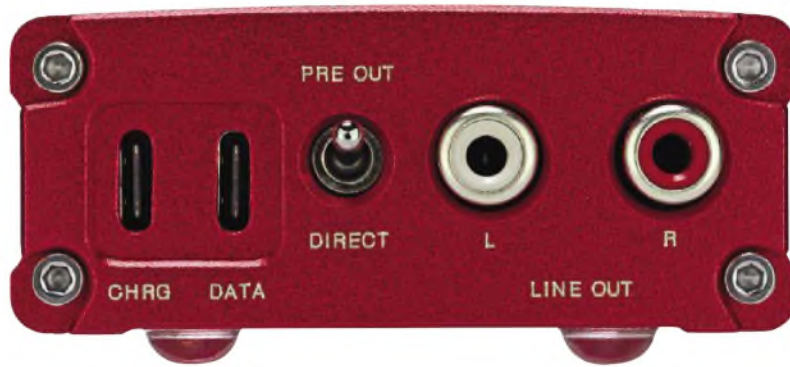
At far left are USB-C ports for charging and data input. A toggle switch selects DAC out (fixed level) or PRE OUT (variable through volume control). Two RCA phono sockets deliver a line output.
