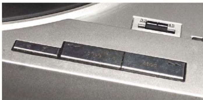
Raising and lowering the tonearm is by push-button at left. At right are the start/stop buttons that, with the arm raised, double as two-speed manual track-seekers. As with the SL10, the 33/45 speed switch is under the cover.
