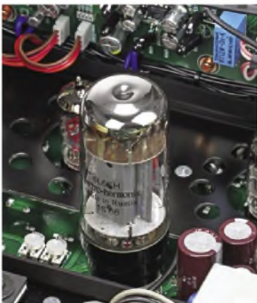
A 6L6 output valve, sitting in a printed circuit board mounted ceramic socket – a common arrangement in modern valve amplifiers.
