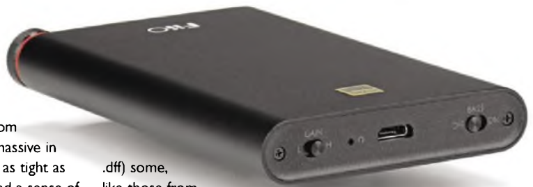
The bottom face carries a microUSB input socket and small slide switches for adjustment of Gain and Bass.
