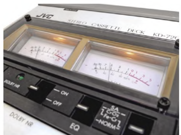
One of the best features of this modestly-priced deck is the backlit metering, readable thanks to its angled 'wedge' design.
