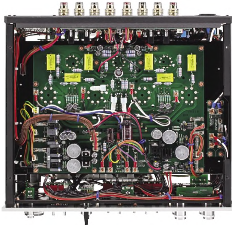
Our underside view shows large yellow high-voltage film capacitors and large resistors typical of valve amplifiers. Switching is carried out by sealed small-signal relays.
