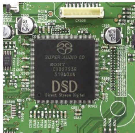
Look at all the feet sticking out. This isn't a millipede but a complex Sony DSD processing chip with arrays of connection points.
