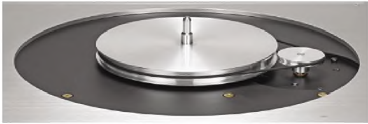
A machined zinc hub with press-fit bearing is driven by a closely sited synchronous a.c. motor. The belt is specially ground T+A say (i.e. not a cheap rubber O-ring).
