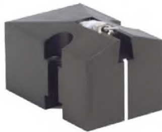
Denon's renowned DL-103 budget moving coil cartridge; it has a spherical stylus.
