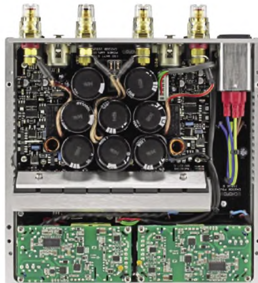
The upper section of the internally-busy TToby is dominated by the amplifiers and a collection of smoothing capacitors. Beneath is a heat sink for the output devices. At the bottom are two fan-cooled (quiet!) switched-mode power supplies.
