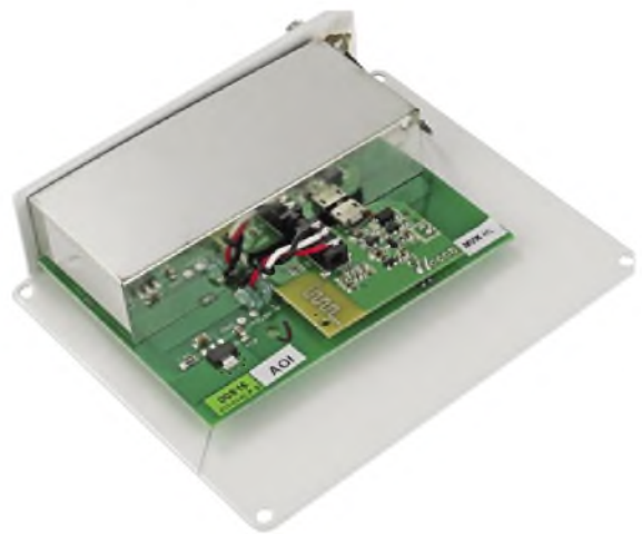
The inside of the Pro-Ject Phono Box BT E. A metal box shields its sensitive analogue electronics to interference from the Bluetooth radio transmitter. It interfaces to the phono stage via three wires soldered to a 3.5mm socket.
