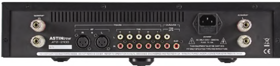
There are five RCA inputs as well as balanced XLRs, and pre-amp and sub-woofer outputs.
