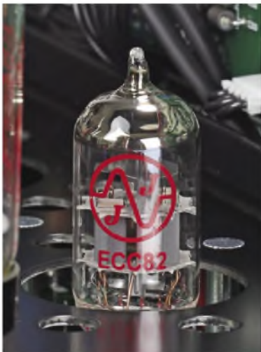
One of the ECC82 small signal preamplifier valves, also used for phase-splitting. Valves like this have a long life of around 10,000 hours.
