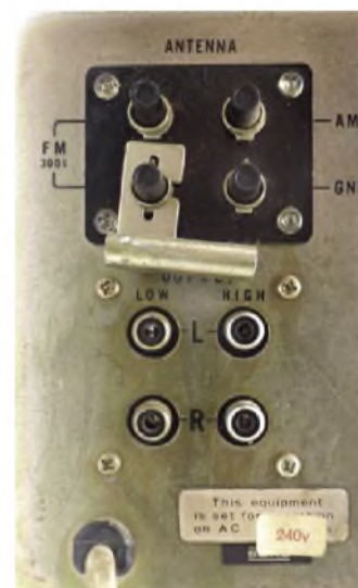
To enable a good match to the rest of your system, the ST-80F offers separate low-level (770mV/10k) and high-level (2V/10k) outputs. They can be used simultaneously – a tape deck and amplifier without tape-loop can both be connected. Separate AM and VHF/FM aerial terminals are provided. The latter has a 300-ohm impedance, meaning that a 'balun' transformer is necessary for some external aerials
