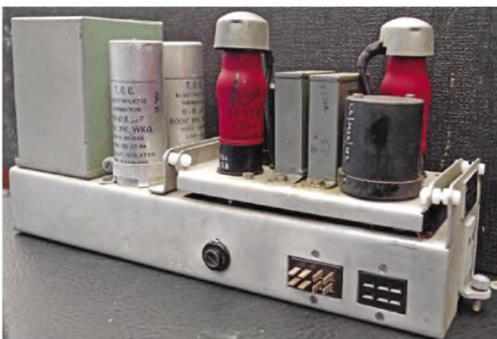
The valve amplifier is sturdily built and uses EF37 pentode valves (red) fitted with top caps that carry a high and dangerous anode voltage. At left sit tall tubular high voltage capacitors that were left in place, but bypassed by modern types.
