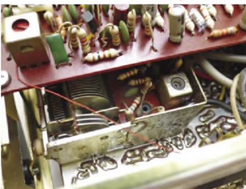
Part of the ST-80F's tuner 'front-end', this truly 'old-school' 5-gang (3 FM, 2 AM) variable-capacitor is a physically-smaller version of the sort of component you would find inside a 1930s 'steam radio'. Within this unit, there's not single varicap diode or frequency-synthesiser chip – much cheaper-to-make parts that are essential to more modern digital tuners.
