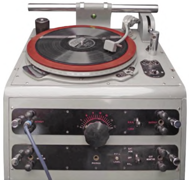
The pickup arm carries a sturdy EMI Type 12 cartridge. It is lifted and lowered by a massive lever at rear right.
