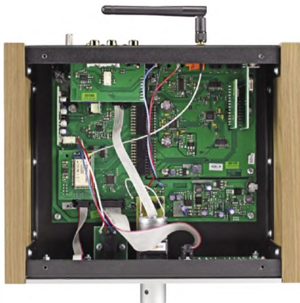
The Pre Box DS2. Its modularity, which aids upgrading and repairs, is evident. Note the screened Bluetooth module and motorised ALPS volume control.
