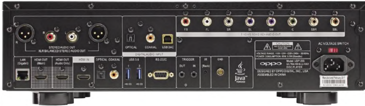
The Oppo's busy rear panel includes both balanced and unbalanced outputs (left) as well as optical, coaxial and digital inputs, plus USB. There's also facilities for multi-channel output for surround sound.
