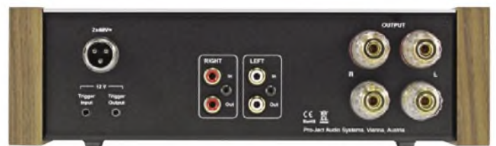
The phono socket inputs (and DC standby trigger) are accompanied by loopthrough outputs and decent speaker terminals. Note that the power supply is external.
