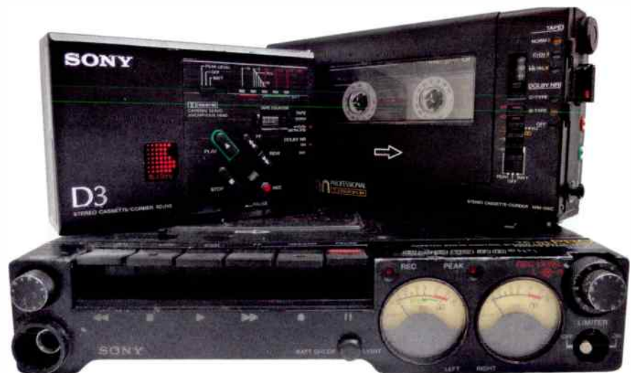
Sony's top portable stereo cassette decks grouped together. To the left of the WM-D6C is the WM-D3. This less expensive Walkman Professional option is about the same size as a play-only Sony unit of that time and uses a very similar mechanism. Like the bottom machine that dwarfs both - a compact (but non-Walkman) TC-D5 Pro portable used by BBC TV in the early 1980s - the WM-D3 is capable of making decent recordings.
