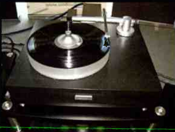
This is the Bergmann Sindre Airbearing turntable fitted with their linear tracking airbearing tonearm. www.bergamnaudio.com
