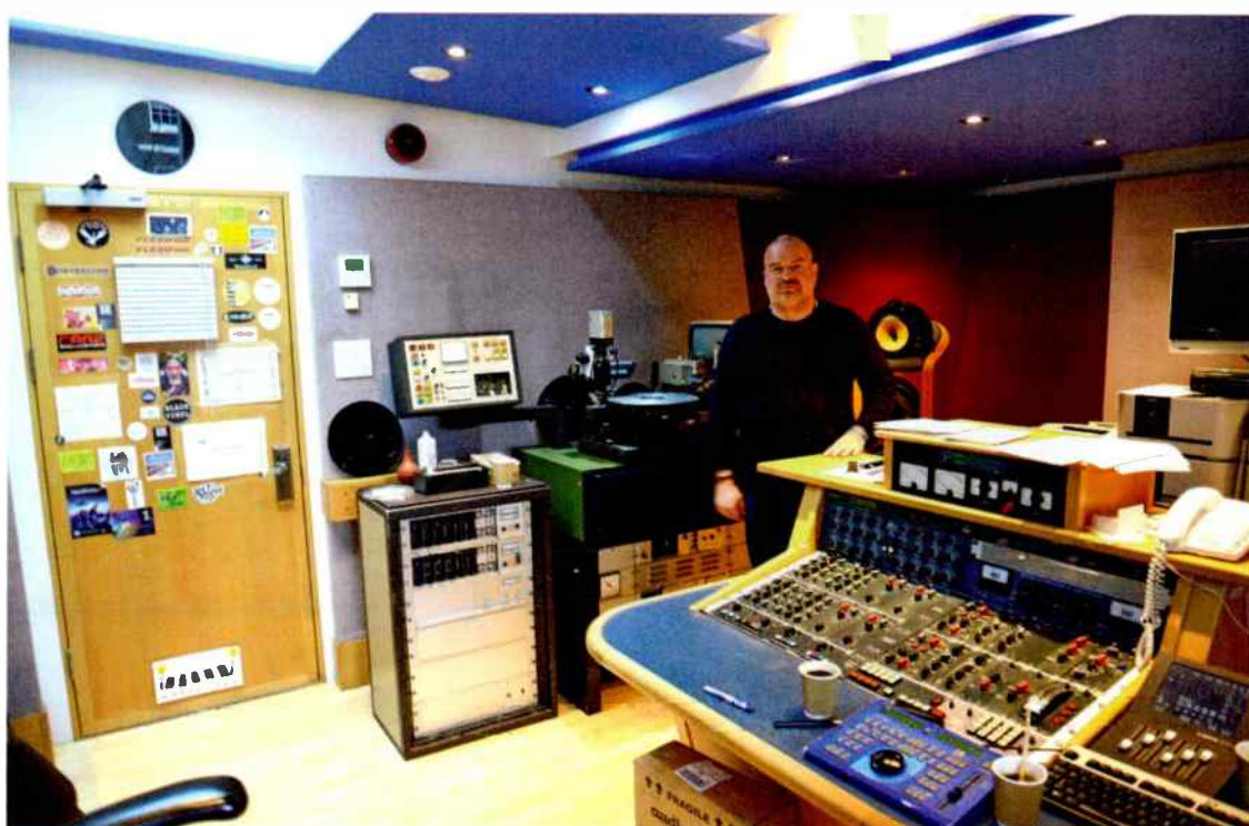
At left of cutting engineer Sean Magee is the Neumann VMS80 lathe with SX-74 cutter head, used to cut the latest mono LPs. In front is the mixing desk and behind him a B&W 800D studio monitor.
