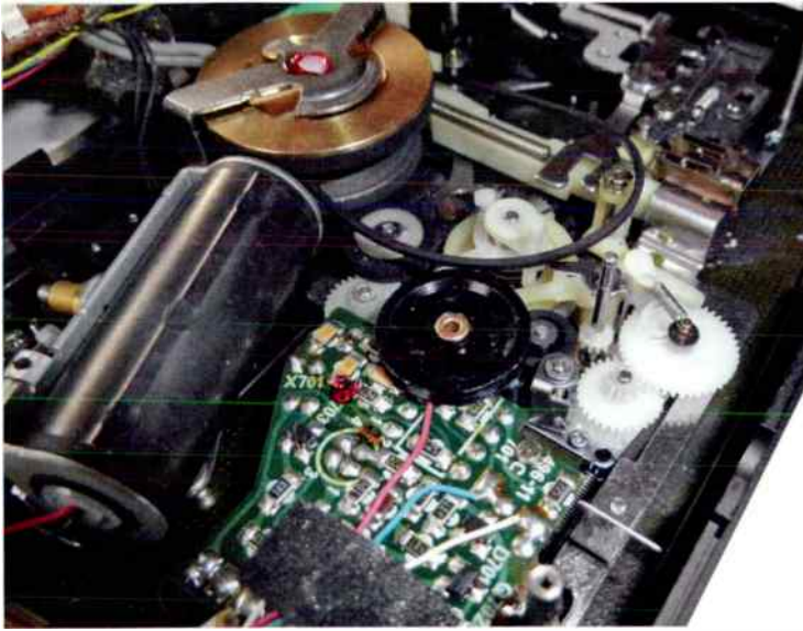
What you'll see if you strip down a WM-D6(C) mechanism. Here we see the motor, which couples the brass flywheel via Sony's 'disc drive'. The belt drives the cassette's takeup or feed reels.
