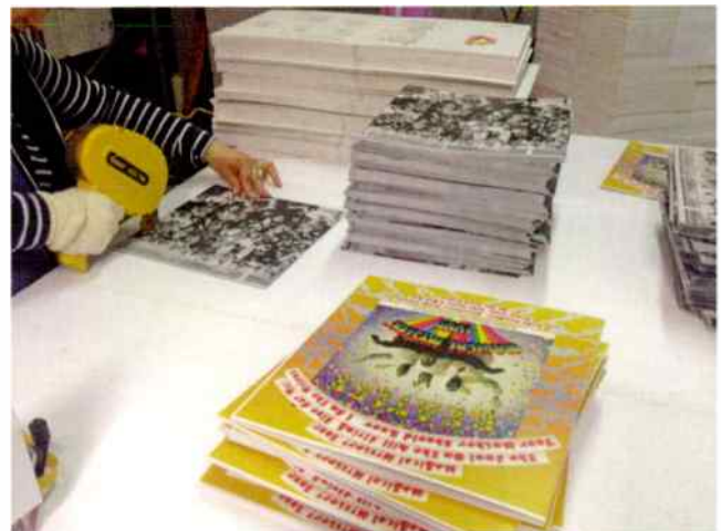
LP production at Optimal Media, Robel, Germany. Clean conditions are used to avoid dirt and fingermarks.
