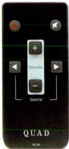
The simple remote controls volume and input. Volume level is shown by yellow LEDs on the Master loud-speaker.
