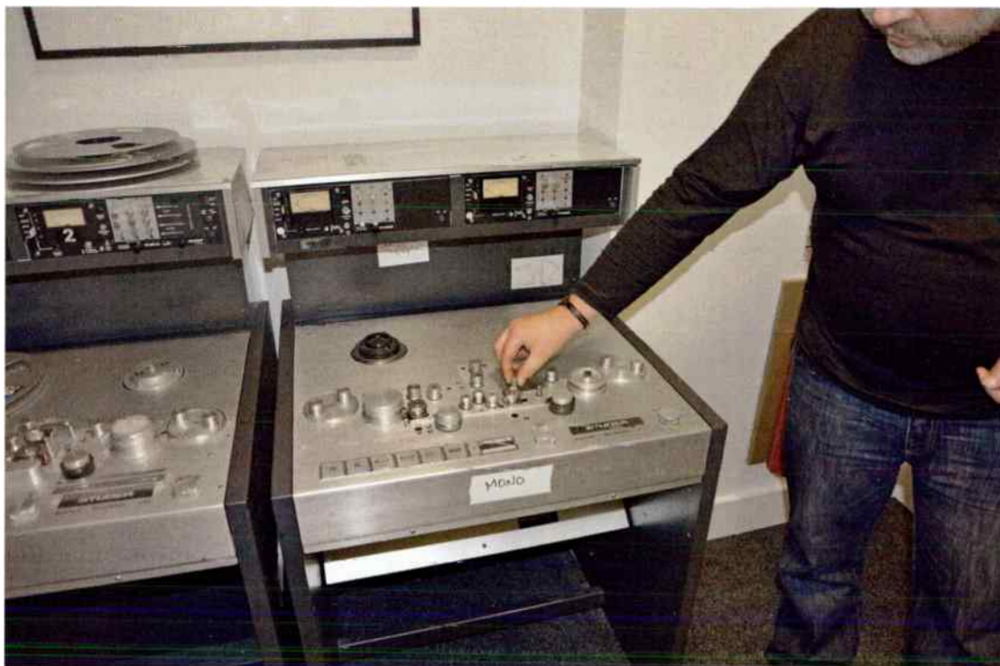
The Studer A80 tape recorder with mono replay head used to re-run the mix-down master tapes. Sean Magee fingers a specially fitted manual azimuth adjustment control to ensure the replay head aligns with the tape's recorded azimuth.
