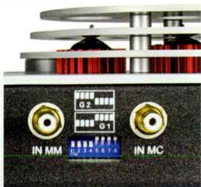
Each channel is equipped with dip switches to set G1 or G2 levels of gain.
