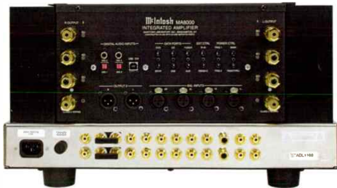
Balanced analogue inputs and outputs through XLR sockets on the rear panel, massive loudspeaker terminals, and digital connectivity, including asynchronous USB.
