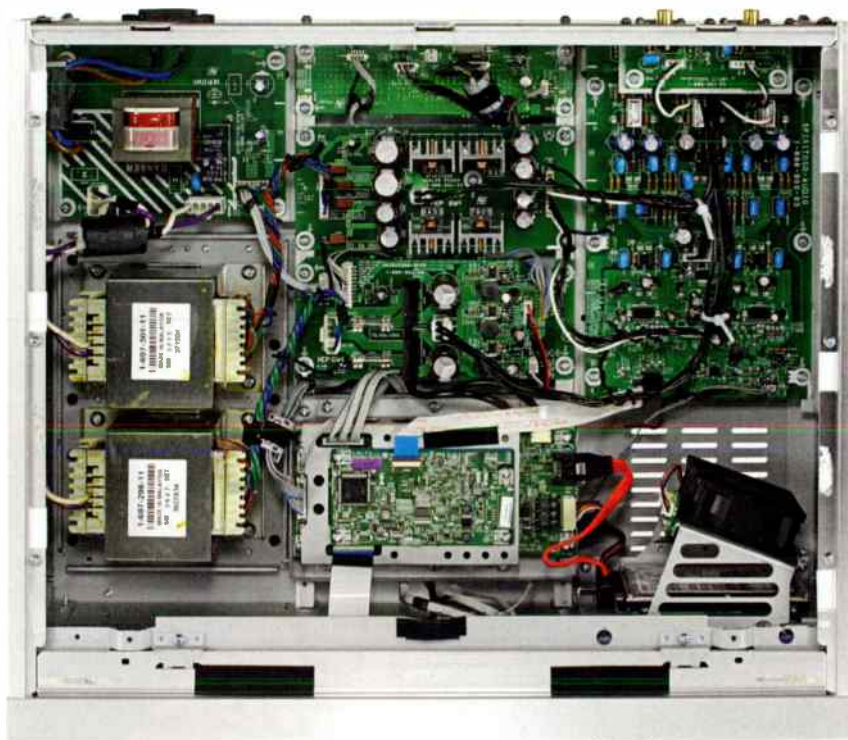
Inside the large chassis sit three mains transformers (at left), explaining the player's weight. Independent power supplies provide isolation between analogue and digital, improving sound quality. Sony told us a Burr Brown PCM 1795 DAC is used.
