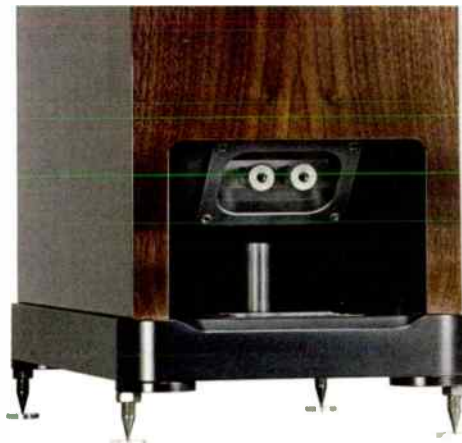
A twin venturi floor port with central aerofoil section smoothes and damps the bass cabinet. Our measurements show it was effective in improving bass damping.
