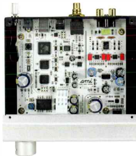
A packed circuit board, complete with top Cirrus CS4398 DAC.
