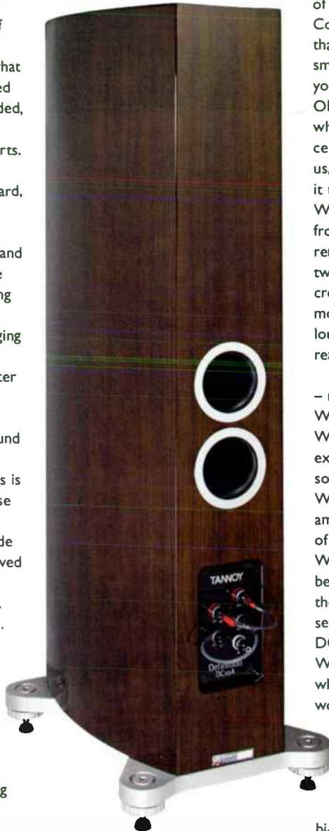
The rear panel carries sturdy WBT loudspeaker terminals and an earth terminal too.
