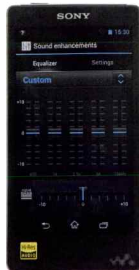
A five-band graphic equaliser and 'Clear Bass' slider can modify sound quality.
