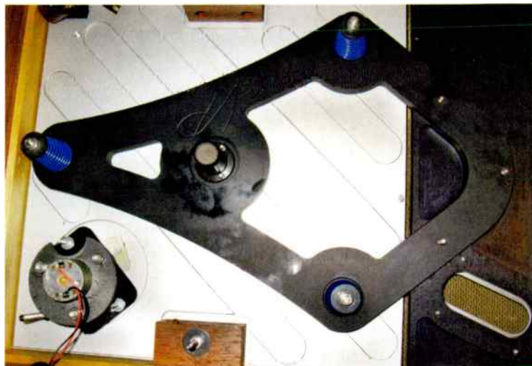
"The Unity 2 armboard and chassis fitted to my Sondek prior to fitting the arm and setting the bounce. My oily paw prints are yet to be wiped off the subchassis!"
