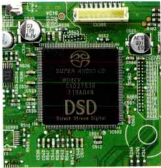
Sony's CXD2753R chip retrieves the DSD datastreams from an SACD disc and sends them to the DAC (ESS Sabre ES9016).
