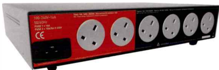
The two sockets (16Amp) in the red coloured area are for high power components such as amplifiers, while source components use the four lower power (10Amp) sockets in the black section. The IEC mains input is on the left.”
