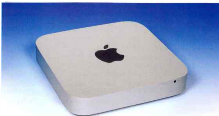
A Mac Mini can be fitted with a Solid State Drive (SSD) and is a popular music server, due to small size, silence and an operating system that is compatible with high-resolution digital.
