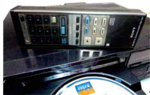
Very much a deluxe item. This full-function infra-red handset could operate all of the CDP-101's key functions from the comfort of your armchair. We take such convenience for granted today, but the CDP-101 was the only first-gen CD player to offer remote control as standard.
