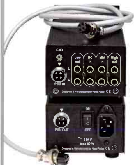
Rear carries phono socket connections only, not XLRs.
