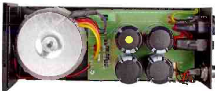
Power supply has a toroidal transformer and big smoothing capacitors.
