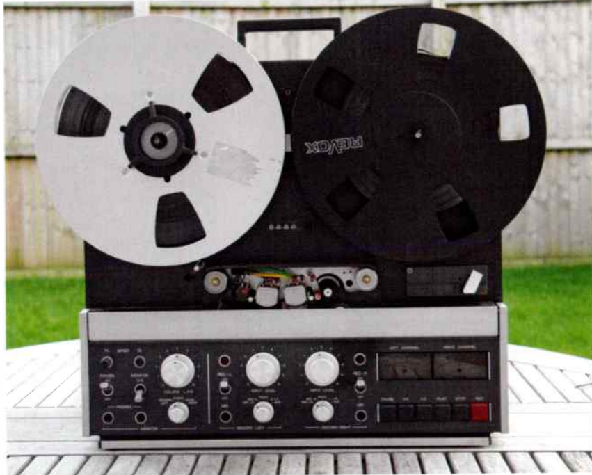
B77 in all its glory, note NAB reel to left, Cine reel to right.
