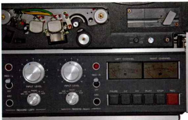
Variable speed and tape editing block, main differences between MkI and MkII
