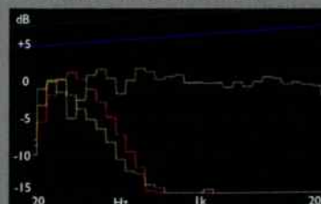
Green - driver output Red & Yellow - port output
