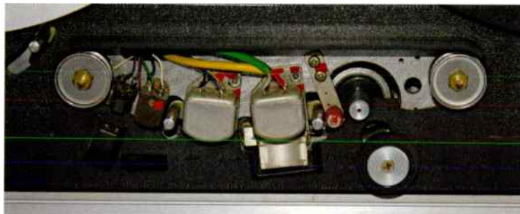
Head block front and back, star 'REVODUR' heads make the big difference from A77
