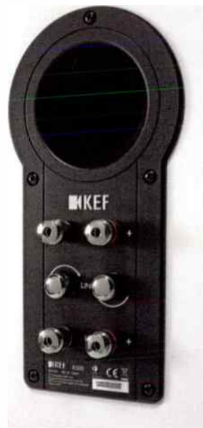
No bi-wire links to lose: just unscrew the internal links.
