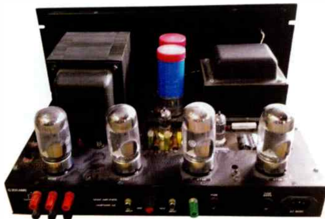
A Grant 200 tube amplifier uses four output tetrodes in fixed bias to deliver high power, but was for the U.S. market.
