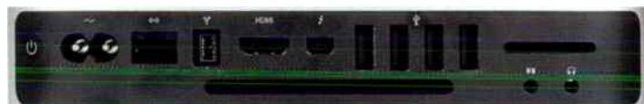
Spot the audio sockets! The traditional ones are at far right, a 3.5mm analogue microphone input and a headphone output that doubles as an S/PDIF optical digital output. The USB, HDMI and Thunderbolt outputs can stream digital audio as well.
