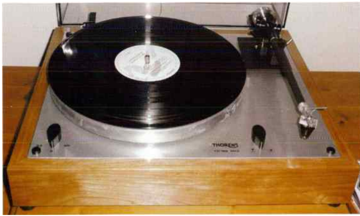
The Thorens after its rebuild, with cherry plinth and Inspire X100 arm, fitted with an Ortofon Black MM cartridge. This little lot will give a great sound.
