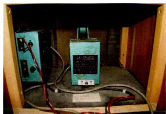
Rear cabinet view. Small power supply on left, back view of tweeter. Crossover on cabinet back.
