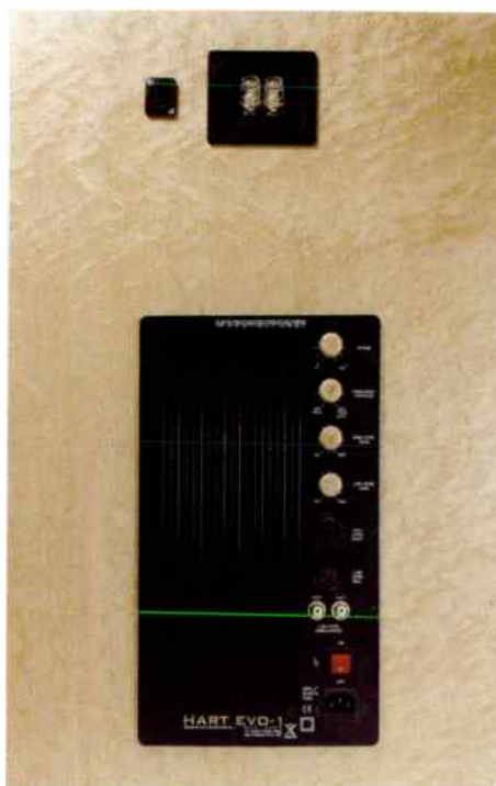
Rear of the main cabinet, showing heatsink of subwoofer amplifier, and its controls...
