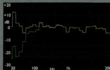
Green - main driver output Yellow - driver+sub output
