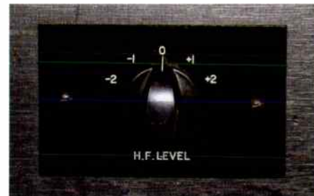
User adjustable levels on back panel, direct to crossover printed circuit board.
