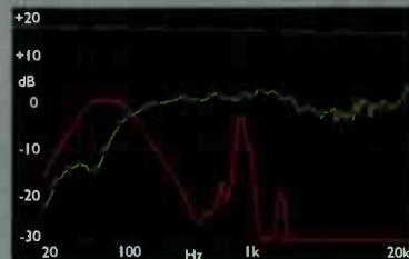
Green - driver output Red - port output
