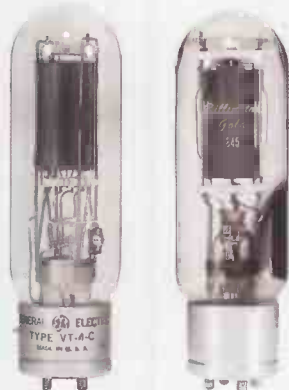
Radio stars - the tall 211 (VT-4C at left) and squatter 845 both provide superb sound quality.
