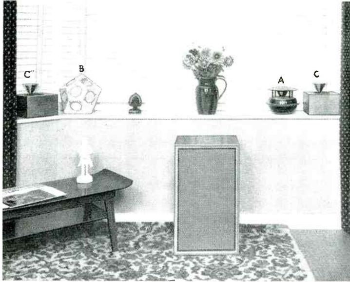
Fig. 10/7. One bass speaker and various treble units. A Goodman's Bowl. B Multi-speaker array for wall mounting. C 5" unit with diffuser.
