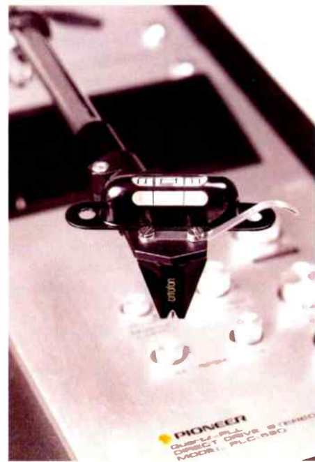
The spirit level is placed on the headshell to enable precise angular adjustment.
