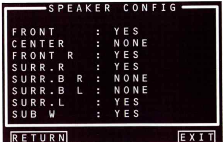
Menu with None. Most quality A/V receivers will feed the Centre Channel into Left and Right if you select NONE for the Front Centre loudspeaker during Setup. This eliminates the Centre loudspeaker altogether, giving normal frontal stereo.
