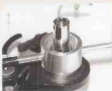
Inside the unipivot showing the dashpot...
