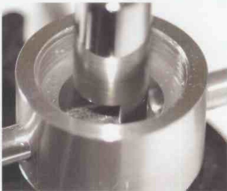
Believe it or not, the new wires will have to negotiate this 90 degree bend around the dashpot!
