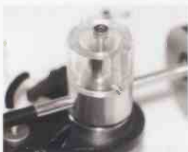
Close-up of the unipivot assembly.
