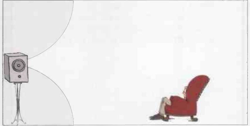
Lifting the speaker on a stand or shelf reduces its ability to couple into the first vertical room mode.
