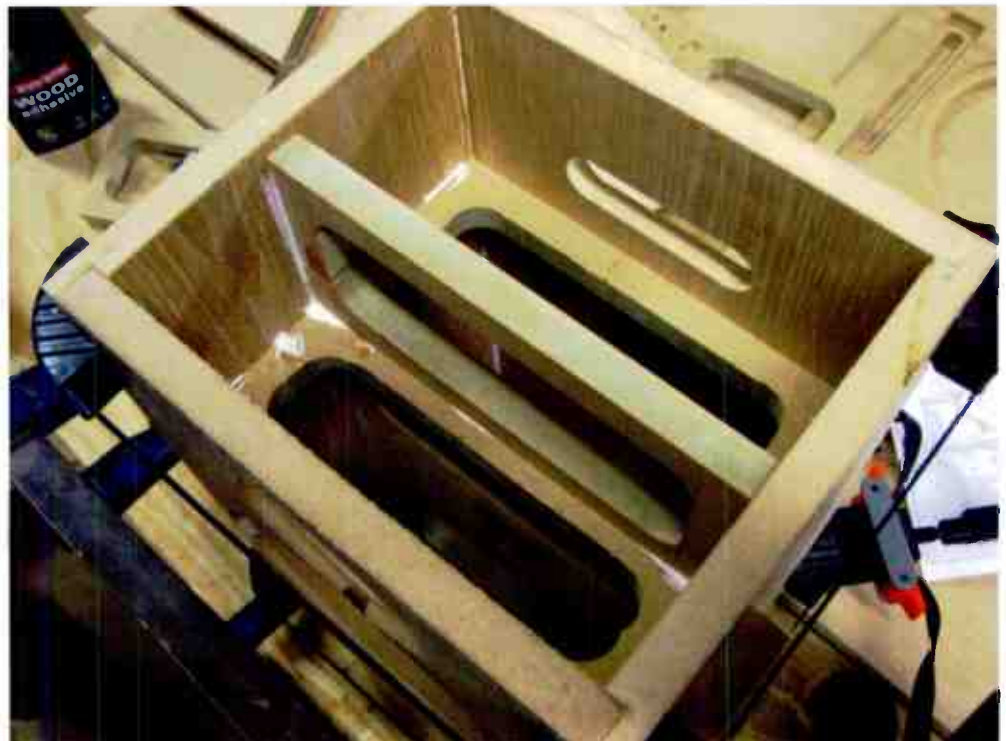
Watching glue dry! A top view of the internal baffle arrangement, showing vertical brace position.
