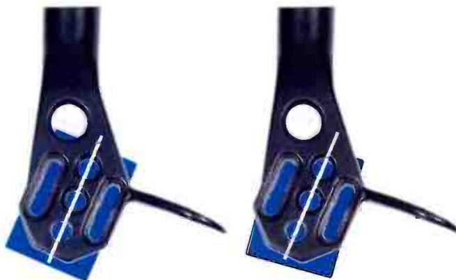
Misaligning a cartridge in the headshell by a few degrees significantly increases tracking distortion. At left the cartridge body is in alignment with the headshell axis. At right we show a 5 degree error - small in visual terms but large in its affect upon performance.
