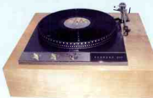
Garrard 401 bolted straight into solid plinth. Derived from the 301, it was intended for heavy duty use in studios and the like. Decks like this are very easy to use, as in heavy plinths they are very steady.
