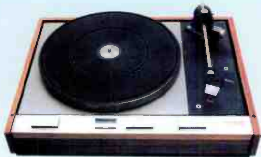
Thorens TD125, an early suspended sub-chassis turntable. The platter and arm float on a spring suspended sub-chassis, for isolation from vibration. Chassis bounce makes arm cueing a little difficult.
