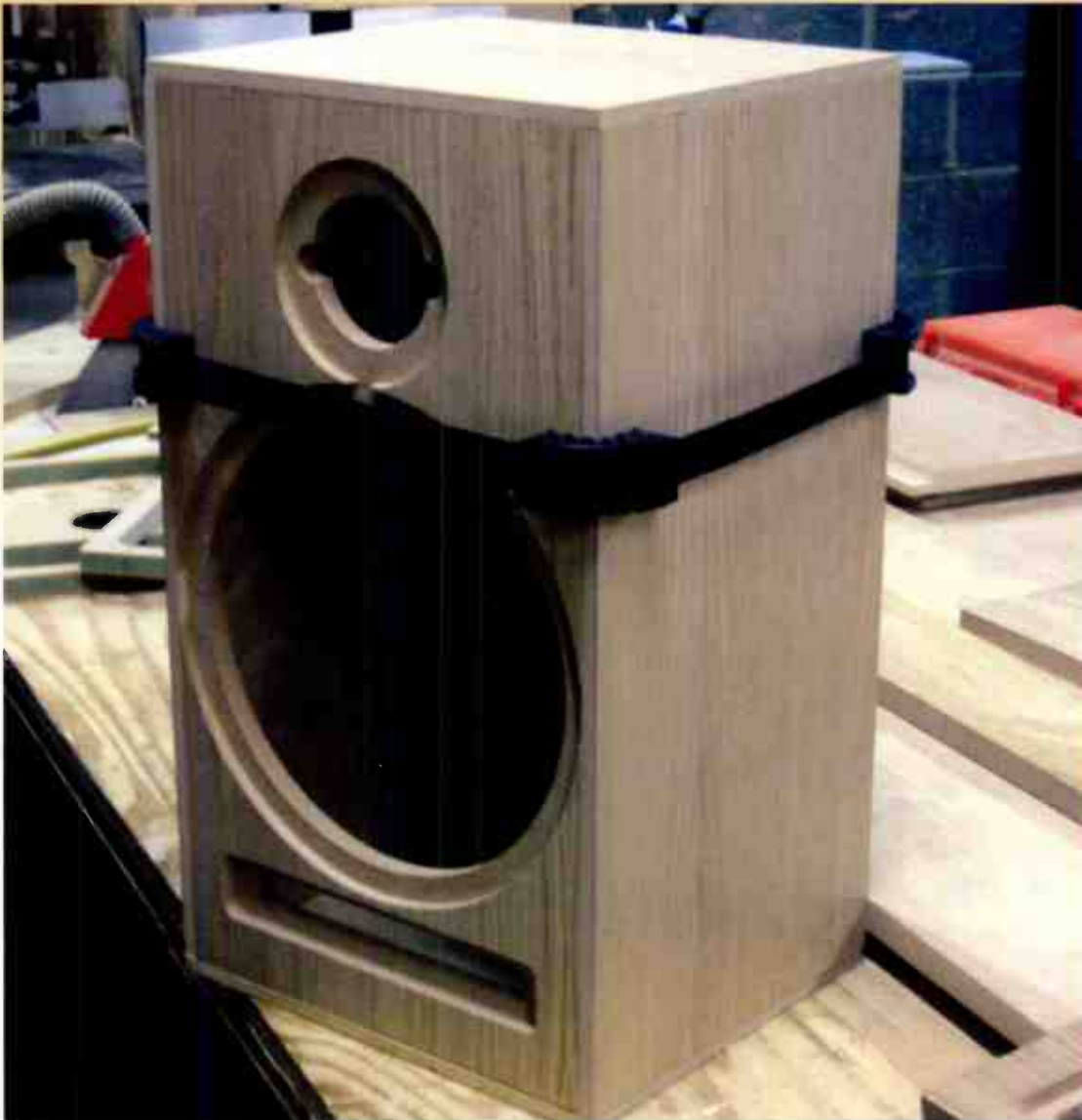
Final cabinet assembly, with strap to hold cabinet whilst glue dries.
