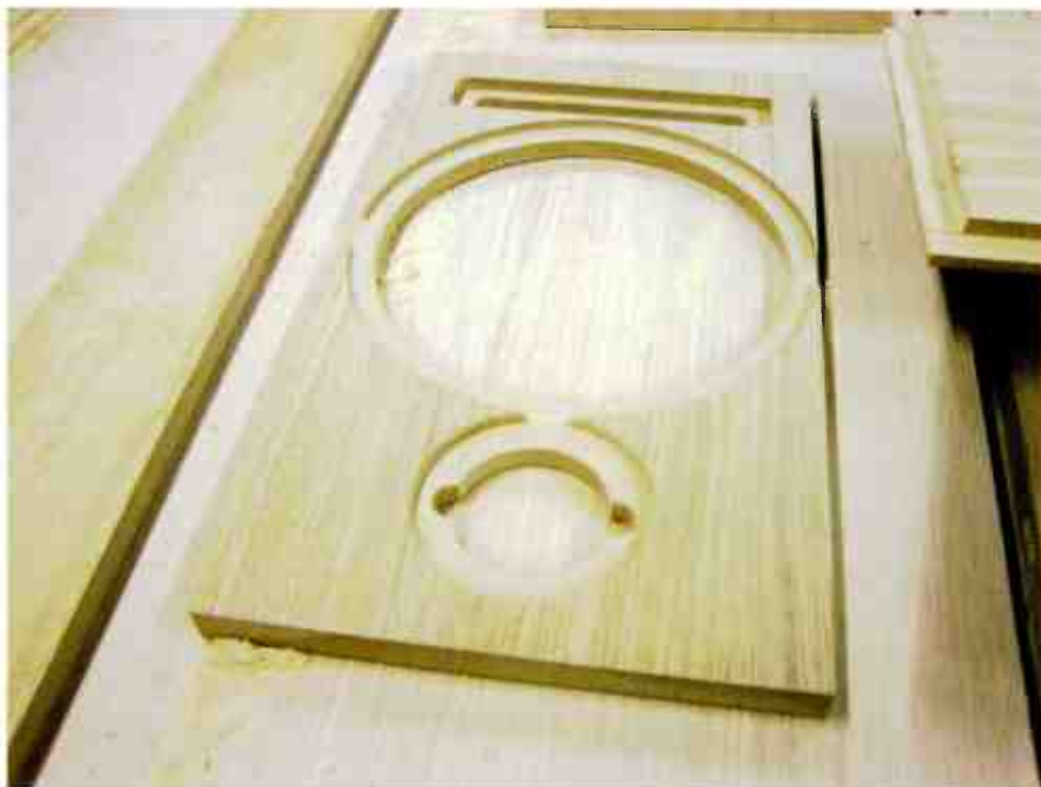
Front side of front baffle, with routed cutouts for flush fitting of drive units.
