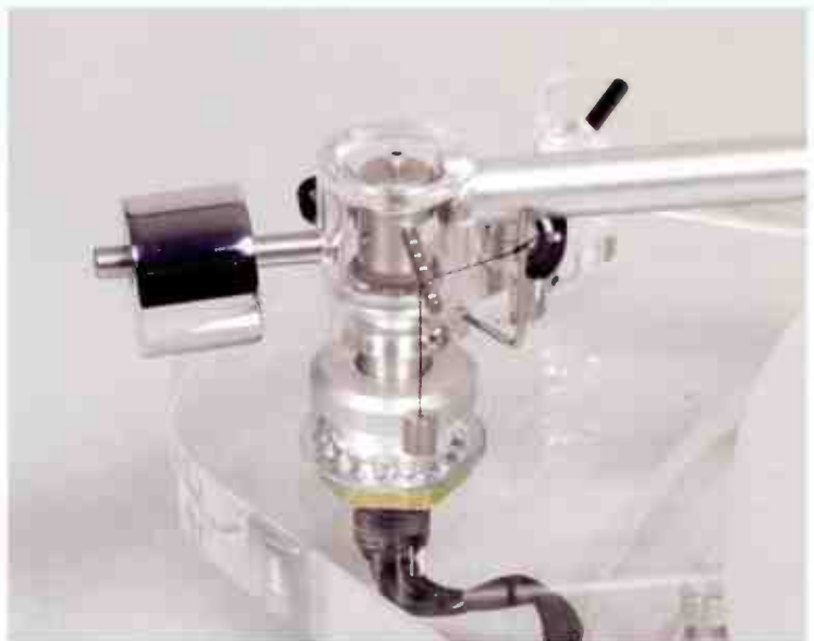
Weight and thread bias force mechanism of the Roksan arm. It applies an outward force to counteract to natural inward force that arises from an offset headshell. Other methods are springs and magnets. Bias improves tracking. Experiment to get the most stable sound.
