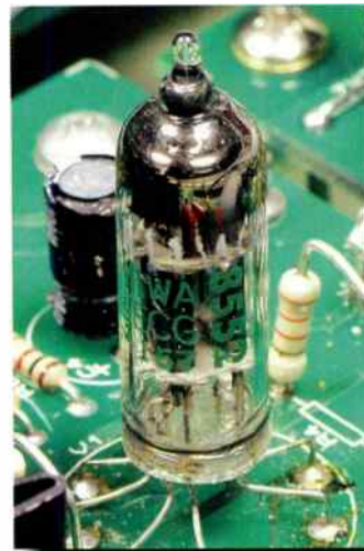
The QC-twenty four's wire-ended Philips 6111WA double triode valve. Originally for military use, like sitting atop an ICBM, it is rugged.
