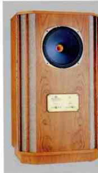
Fig. 4 Big loudspeakers go loud. This is the recently introduced Yorkminster from Tannoy, standing over one metre high and 600mm wide (2ft) wide. Tannoy claim sensitivity of this big reflex is 94dB. Our chart shows it needs 4W or so to produce 100dB!
