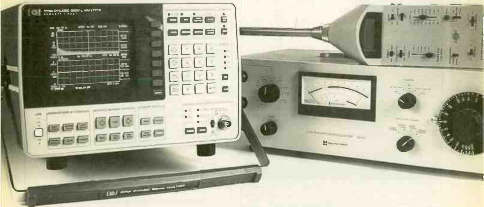
PRODUCTS ARE TESTED USING FFT SPECTRUM ANALYSIS APPLIED BY A HEWLETT PACKARD 3561A, AT LEFT HERE. AT TOP RIGHT IS OUR BRUEL & KJAER SOUND PRESSURE LEVEL METER WITH MEASURING MICROPHONE, AND BELOW A LOW DISTORTION RADFORD SINE WAVE GENERATOR.
