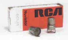
tional valve: no top supports in the form of mica discs; no 'getter'; no glass envelope to melt. At the time of their development it was hoped that power Nuvistors of about 30 Watts would not be long in arriving. What could be more perfect!
