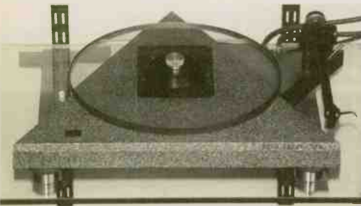
Like Pink Triangle's Tarantella, Nick Daker's heavily-modified Rega Planar 3 uses a triangular base, in this case supported on squash balls.
