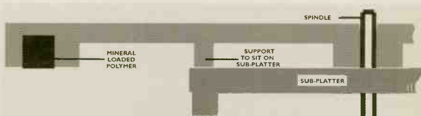
A platter with most of its mass concentrated around the outer edge will aid speed stability in a turntable.
