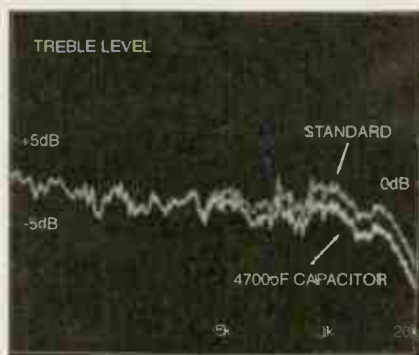
Fig.7 - Output from the HD3P tweeter can be rolled off progressively by connecting a 4700pF capacitor across the tweeter.
