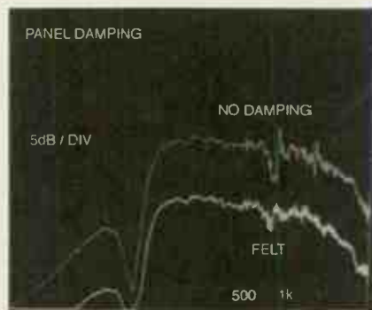
Fig.6 - The effect of carpet felt upon internal reflections. The notch around 700Hz is well suppressed.
