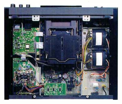
The MDS-JA50ES's transport is much beefier than most MD recorders'. It's also more complex, with its CD-style loading tray. To its left, surface-mount components cover the green PCBs.
