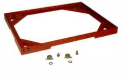
The No Name is one of the simpler platforms here as far as innards go. The outer frame (508mm by 400mm by 50mm) is made from mild steel welded into a rectangle. Four diagonal braces, one in each corner, are filled with SoundBytes (to absorb vibration) and carry the adjustable spikes which sit in brass cups to protect soft surfaces. Four ball bearings mounted on threads allow the glass top-plate to be levelled.
