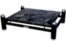
Inside the Monoplinth's hollow steel frame (595mm by 460mm by 180mm) is a mix of small-diameter lead shot and extremely fine casting sand. This is highfrequency agitated, so there are no spaces left inside the frame. The 20mm thick rubber-damped marbleagglomerate shelf is located on four spikes through four small lead decoupling discs. More spikes in the hemispherical aluminium tube ends lift the Monoplinth off the floor.
