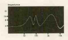
At 89dB the CDM7 is sensitive and will need little power. Unfortunately, the impedance characteristic is one of the most challenging I have seen, swinging from a very low 30hms DCR to over 300hms at 2kHz, vertiginous slopes meaning the load is highly reactive. Amplifier differences will be highlighted. It
