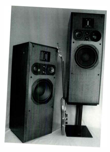
The PLLI loudspeakers use six drivers a side: the famous Tonigen ribbon and two Morel MDT39 dome tweeters, one Morel MWI 14S and one Audax HM100ZO midrange unit, and a Volt B2500.1 woofer. Unlike almost all passive loudspeakers, the PLLIs are phase linear, which benefits imaging precision and overall transparency.
