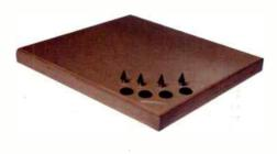
At first sight the Absorber Platform seems like a thick piece of multi-ply wood. Measuring 440mm by 400mm by 36mm it's rather more complicated than it looks. Inside the platform there are 428 individual chambers each of which is 90% filled with small steel balls. The remaining space in the chamber is taken up by fine silica sand.
