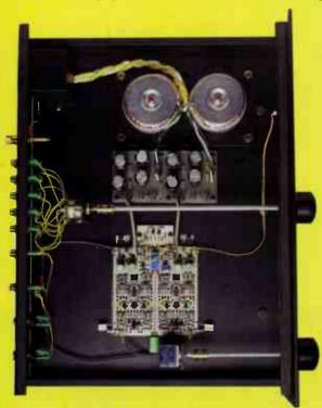
boards. The circuit board itself has a slightly 'homemade' look to it - after all, it says 'Carefully Hand Made By Etalon Ltd in Hungary' on the back panel. Balanced as well as RCA output sockets are provided and volume is controlled by the ubiquitous Alps Blue potentiometer.
